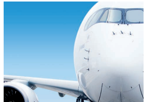
Air-data probes from UTC Aerospace Systems on the Airbus A350 XWB commercial jet supply critical information to the aircraft's flight control and pilot display systems.
