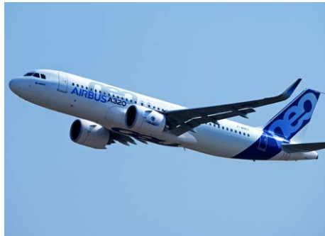
The Airbus A320neo successfully completed its maiden flight in 2014, powered by two Pratt & Whitney PurePower ® PW1100G-JM engines and supported by multiple systems from UTC Aerospace Systems, including nacelles, thrust reversers, electrical power generators, cabin attendant seating, air data sensors, and wheels and carbon brakes.
